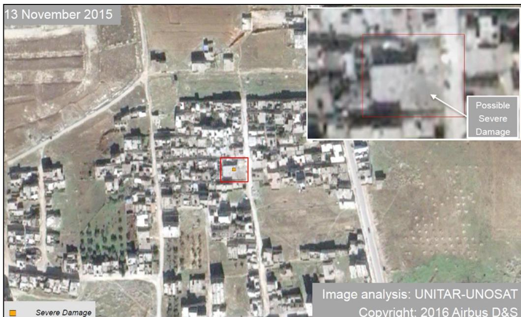
UNOSAT analysed imagery acquired on 13 November 2015 and 15 April 2014 to detect possible damage to the Omar Ibn al-Khattab mosque in Jisr al-Shugur, Idlib. Using satellite imagery based change detection analysis, UNOSAT identified possible severe damage to the main mosque building and probable damage to the mosque minaret.
